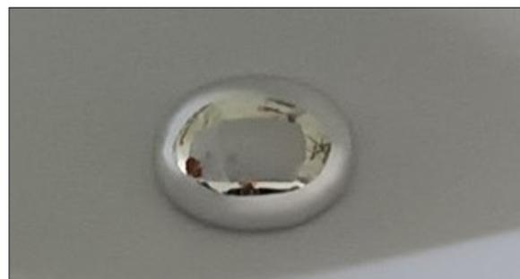
Image of liquid metal after reaction with carbon dioxide in bubble column reactor to form gallium oxide and solid carbon
