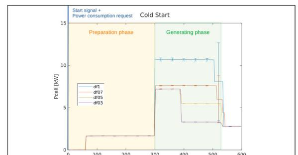
**Power Consumption of the Electrolyzer Cells during "Stand-by Start"**
