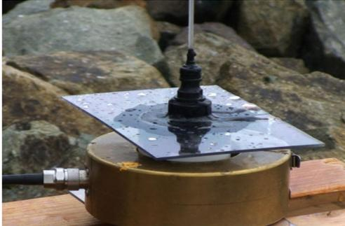
Illustration of the seawater antenna based on design 1, employing a pump and a current-probe.
