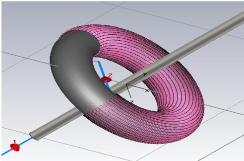
CST simulation model of the current-transformer structure, as it appears in the seawater antenna based on design 1.
