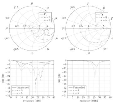
Reflection coefficient of the seawater antennas after impedance matching. Left column: Design 2. Right column: Design 1.
