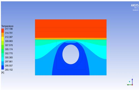
Cross section temperature contour of collector C
