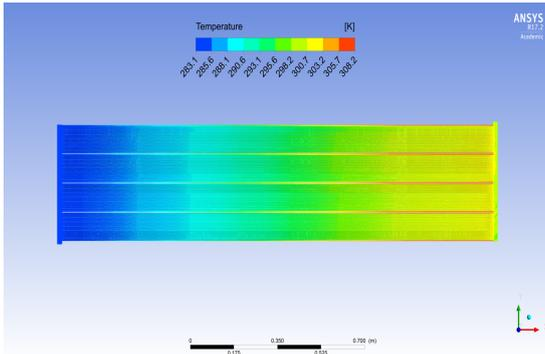
Water temperature contour normal to PVT plane of collector B
