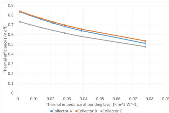
Influence of bonding layer thermal impedance on thermal collector efficiency
