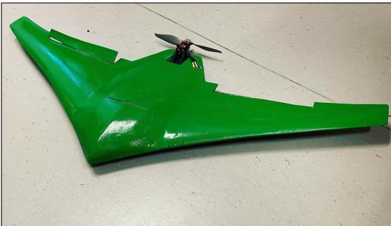
Green Raven GR001 Prototype, a 1:4 scale down of the MK18 kthraero.com/greenraven
