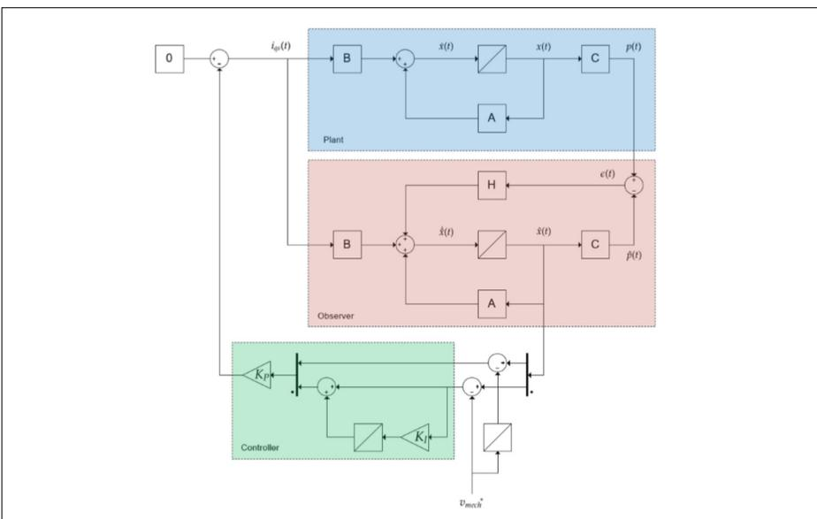
Observer based control schematic
