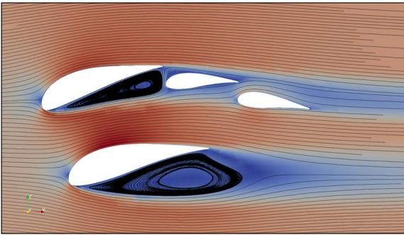
Fig. 1 - CFD Results for Velocity and Flow Separation (AoA = 0°) Own presentment
