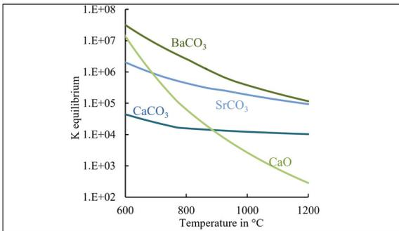
Figure 1: Constant equilibrium for the reaction of barium, strontium and calcium carbonate with HCl over temperature. Own presentation
