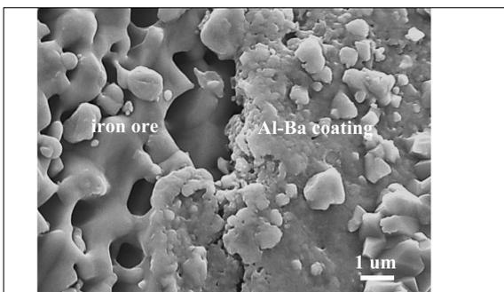
Figure 3: Scanning electron microscopy image of iron ore coated with aluminium-barium after one cycle. Own presentation
