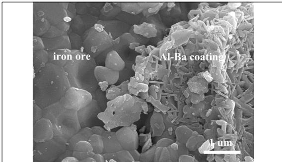
Figure 2: Scanning electron microscopy image of iron ore coated with nanostructured aluminium-barium. Own presentation
