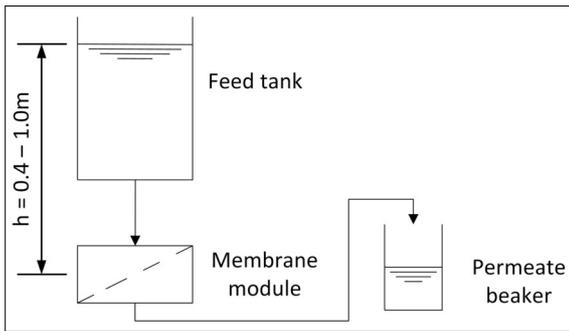
Fig. 1: Schematic of a GDM filtration process
