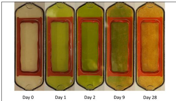
Fig. 2: Cake layer development over time on the UF membrane sheet in the presence of a high concentration of green algae
