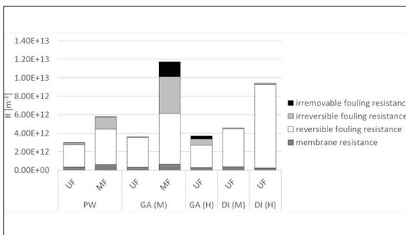
Fig. 3: Resistance caused by the membrane and different types of foulant at the end of the experimental period
