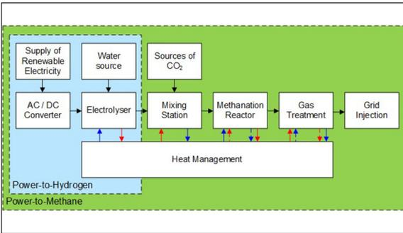
System boundary, Concept of a Power-to-Methane plant
