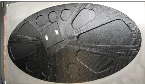
Manufactured disc as sandwich structure with integrated aluminum core for assembly.
