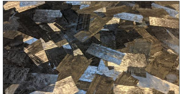
**Material covered with release film after the double diaphragm forming process**
