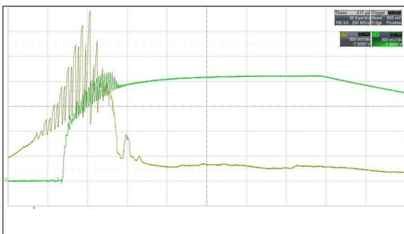
Output voltage (green) versus input voltage (yellow)
