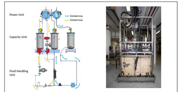
**Charging process: desorption of water vapor from NaOH**
