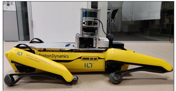
**The robot SPOT with a herbicide sprayer Add-On**
