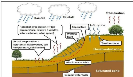
Figure 1: Mechanism of rainfall-induced slope failure
