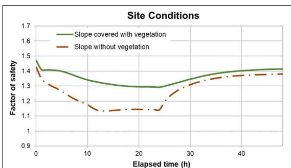
Figure 3: Factor of safety - Elapsed time, rainfall 22 mm/h for 24 h
