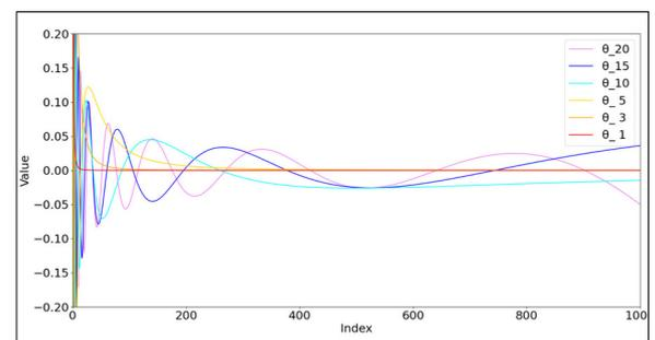
The performance of the wave-filter converges to the one of the Kalman filter.
