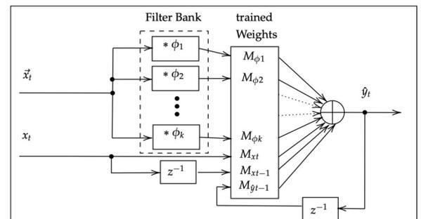
The wave-filters which get convolved with the input signal are the eigenvectors of a specific Hankel matrix.
