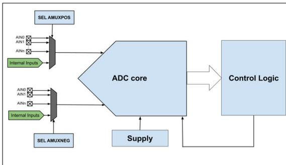
ADC connectivity within the microcontroller
