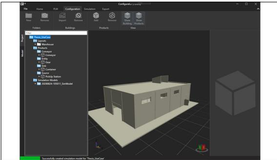
The configurator developed as part of this thesis. The tool loads IFC files and creates a single visualization. Own presentment
